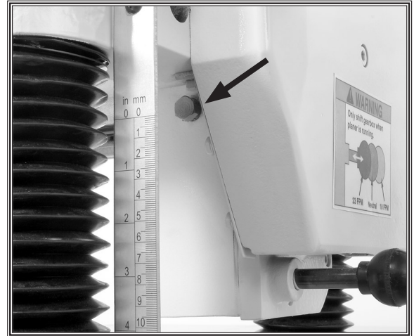
Figure 8. Gearbox fill plug location.
